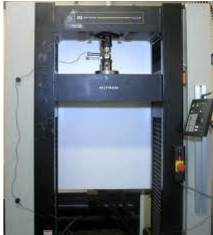
Fig. 2.12. Compression test setup (INSTRON make, 5500R model) used to record stress-strain curves.
