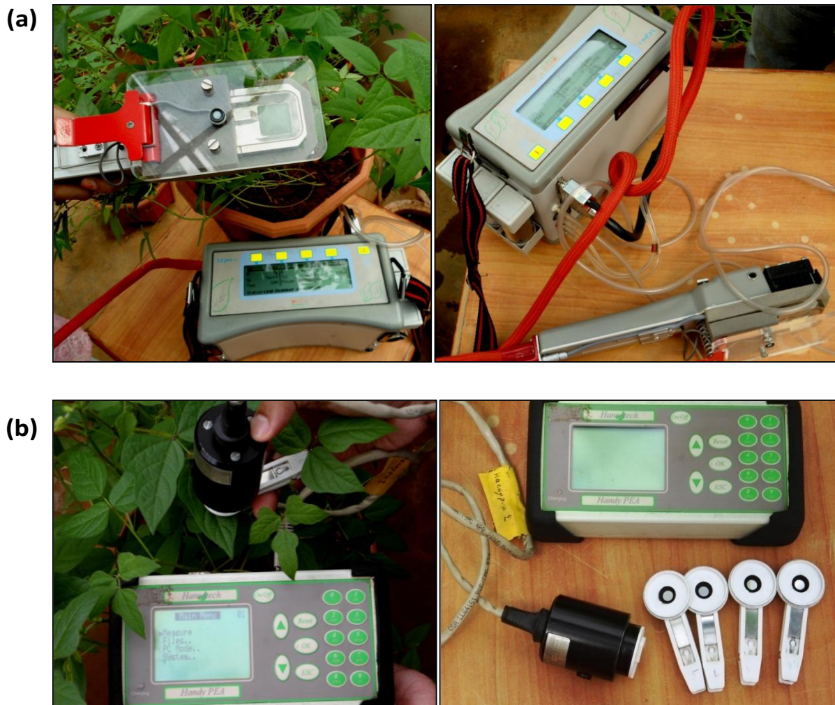
Fig 7. Portable infrared CO 2 /H 2 O gas analyzer, IRGA (LCpro-32 070, ADC Bioscientific Ltd., Great Amwell, UK used for all photosynthetic gas exchange measurements (a). Portable Handy PEA (Plant Efficiency Analyzer-2126) fluorimeter (Hansatech Instruments Ltd., kings Lynn Norfolk, UK used for chlorophyll a fluorescence measurements (b).
