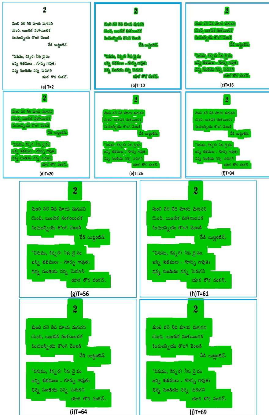
Figure 3.8: Threshold operation on Fringe map of image in Fig. 3.6. (a)T=2,(b)T=10, (c)T=16, (d)T=20, (e)T=26, (f)T=34, (g)T=56, (h)T=61, (i)T=64, & (j)T=69.
