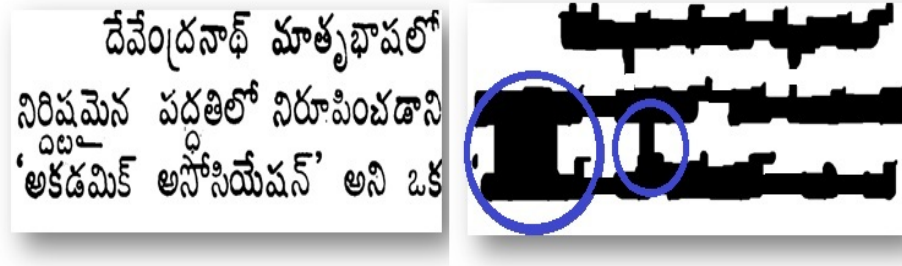
Figure 2.5: Telugu text (left) and Run length smearing (right). Notice that text lines are merged because of consonant modifiers (shown in circle).
