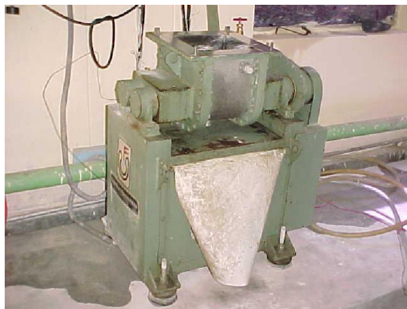
Fig 5.11 Sigma kneader used for dough preparation
