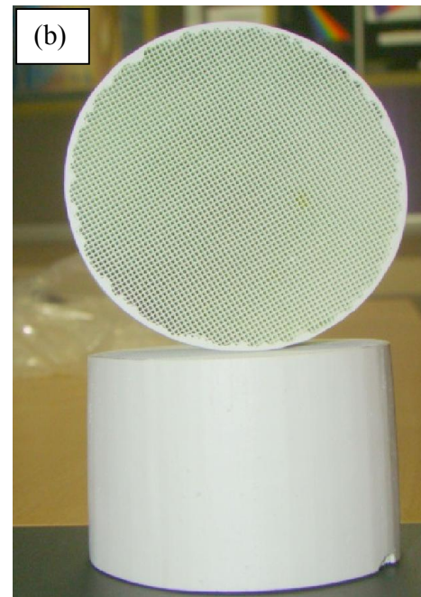
Fig 7 (a) Plot of viscosity versus shear rate of TAT-5 formulation and (b) sintered TAT-5 honeycomb
