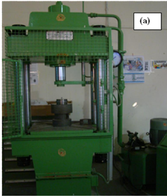
Fig 2.5 (a) Hydraulic press and (b) Green pellets
