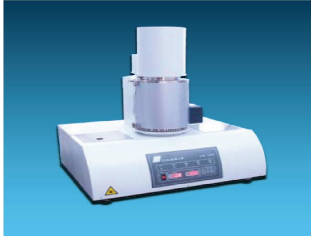
Fig 4.5 Thermal conductivity equipment
