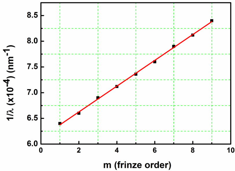
Figure 3.14: Plot for fringe order m vs 1/\lambda for NIR region photonic crystal. Square symbol represents the experimental values and line represents the linear fit based on equation 1.
