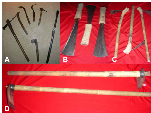
Fig. 6 Use of Melocana baccifera as a handle in agriculture tools. (A) Different agriculture tools. (B) Use of Melocana baccifera rhizome. (C) Combination of rhizome and culm. (D) Use of culm part only.
