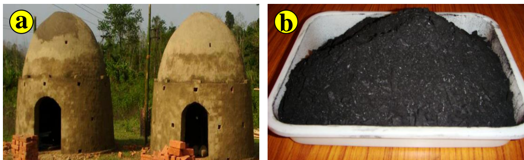
Figure 7. a) Charcoal Kiln from where Melocanna baccifera charcoal is produced and b) Melocanna baccifera charcoal powder after milled with a blender
