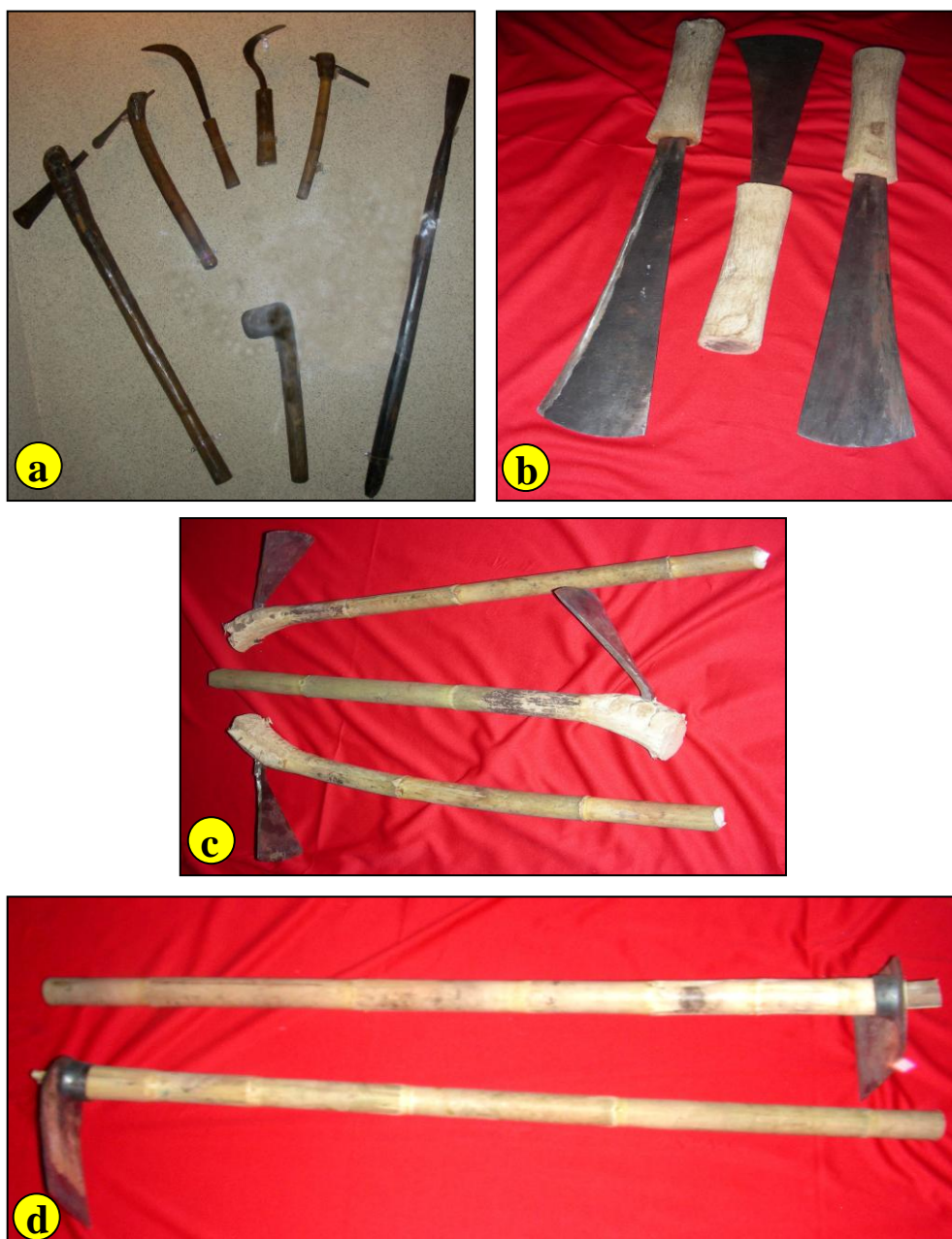
Figure 69. Used of Melocanna beccifera as handle in Agriculture tools. a) Different agriculture tools; b) Used of Melocanna baccifera rhizome; c) Combination of rhizome and culm; d) Used of culm part only
