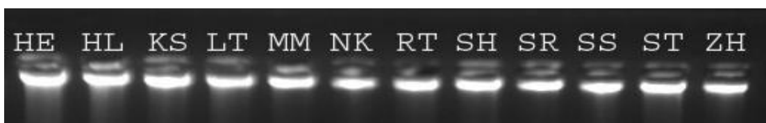
Figure 49. Purified nucleic acids electrophoretically separated on a 0.8% agarose gel for twelve accessions. HE=N.Hlimen, HL=Haulong, KS=Kolasib, LT=Lawngtlai, MM= Mamit, NK= NE. Khawdungsei, RT=Ratu, SH=Saiha, SR=Sairang, SS=Sialsuk, ST=Saitual, ZH= Zohmun
