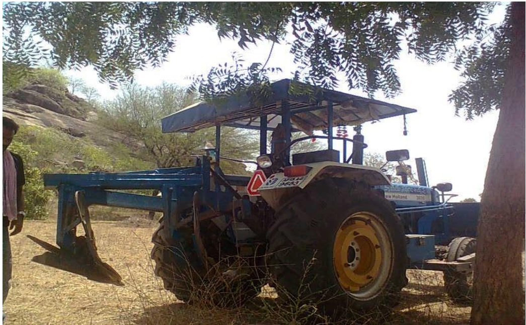
Tractor drawn mould board plough for ploughing
