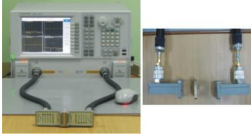
Figure 3.5 Vector Network Analyzer with x-band waveguide adapters and sample holder.
