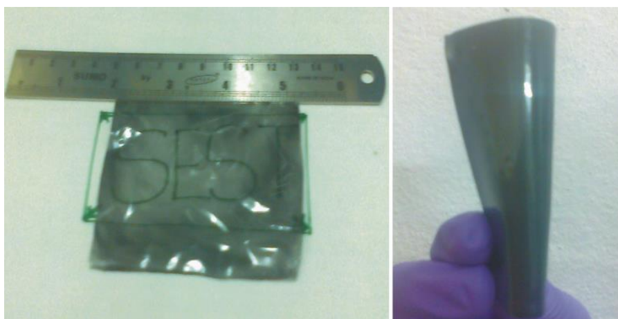
Figure 3.2 Semi-transparent (to visible light) and Flexible 0.2 wt.% FLG/PVA sheet.
