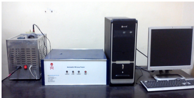
Figure 2.10 Automated P-E loop set up.
