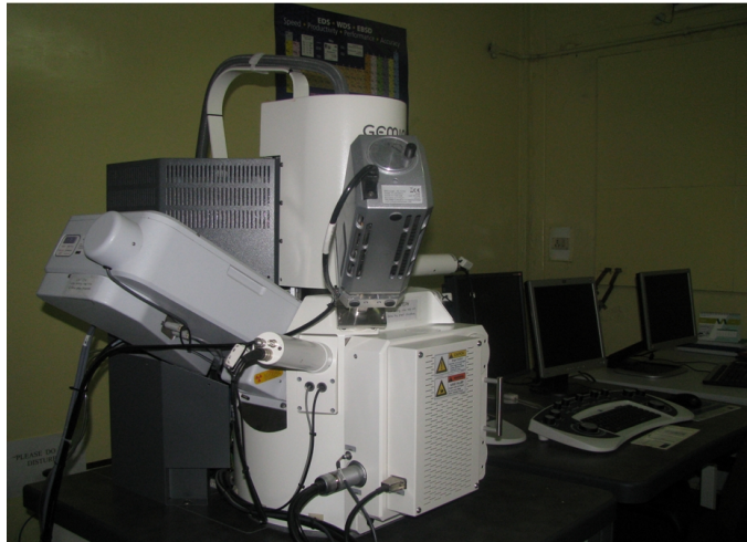
Figure 2.6 Field emission scanning electron microscope
