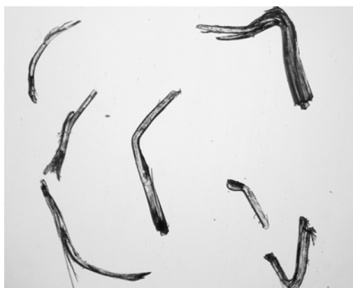
Figure 10. Hexabromobenzene, 3 . Crystals bent into different shapes at 403 K. Photograph was taken after cooling the crystals down to room temperature.
