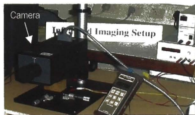
Figure 2.10. Thermal imaging setup
