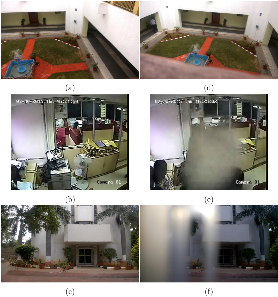
Figure 5.6: Sample frames from our dataset showing visuals of camera tamper events and their intended FOVs in static surveillance systems. (a), (b) and (c) are frames showing intended FOVs. (d) Scene recorded during camera displacement. (e) Scene recorded during camera defocus. (f) Scene recorded during camera occlusion.
