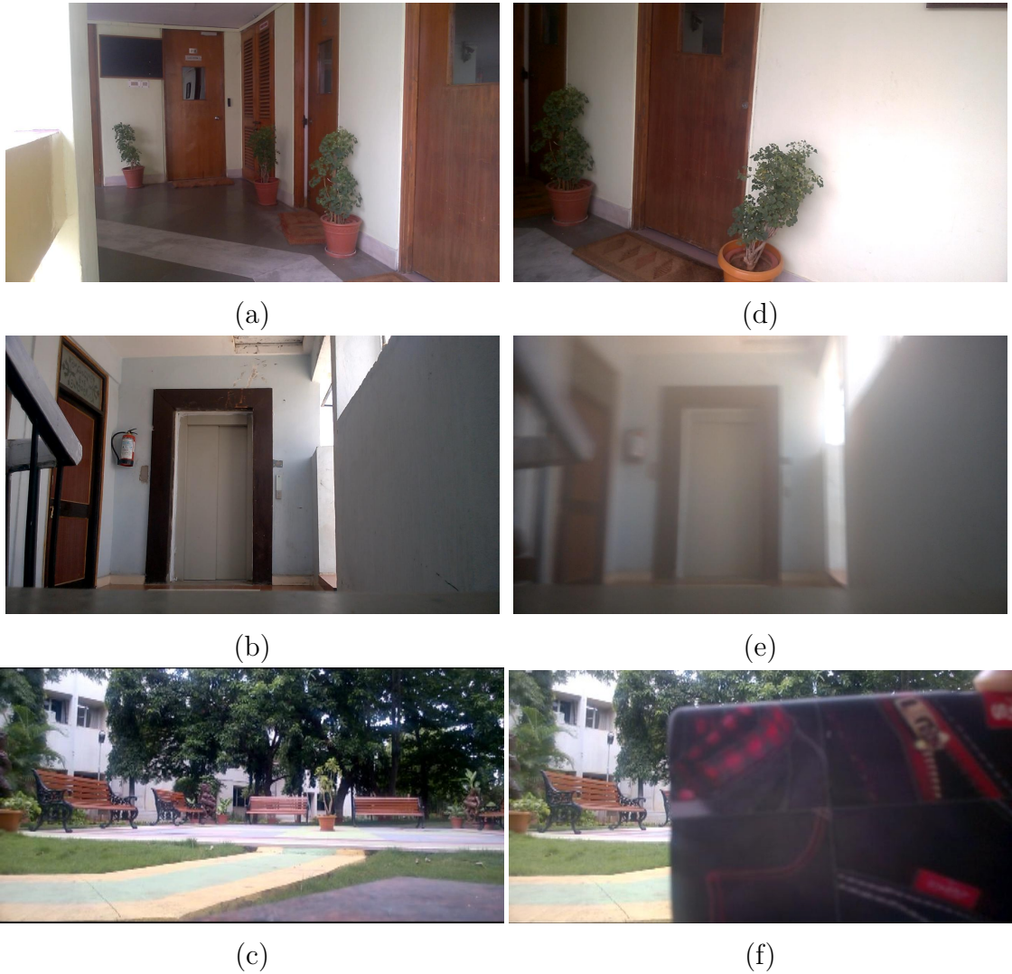
Figure 5.5: Sample frames from our dataset showing visuals of camera tamper events and their intended FOVs in static surveillance systems. (a), (b) and (c) are frames showing intended FOVs. (d) Scene recorded during camera displacement. (e) Scene recorded during camera defocus. (f) Scene recorded during camera occlusion.
