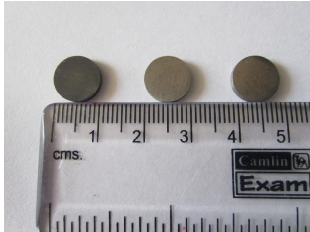
Fig. 8.8 Sintered bulk nc Al-Bi alloy samples.
