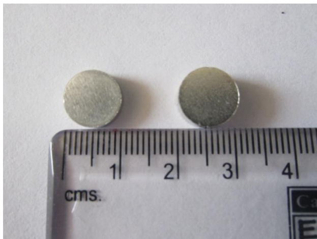
Fig. 4.4 Cold compacted bulk nanocrystalline Al samples.
