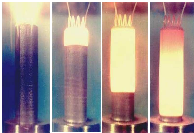
Figure 1.1 Combustion wave propagation captured using photo registration method [38].
