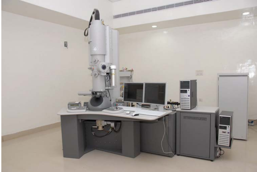
Figure 2.10. Photograph of the Transmission electron microscope (model: model: Tecnai 20 G2 STwin, FEI electron microscope operated at 20 kV using Gatan CCD camera) (established at CFN, UoH) used in the current study.
