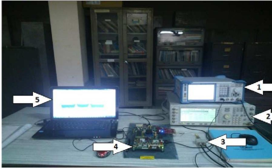
Figure 5.6: Realtime Spectrum Sensing algorithm evaluation Setup : (1) Noise Generator RS SMBV 100A, (2) Signal Generator Agilent 4430B, (3) Pasternak 2000 Power Combiner, 70 MHz BPF (4) Xilinx ML605 with Virtex-6 XC6VLX240T-1FFG1156 FPGA and FMC-150 ADC/DAC add-on card, (5) Simulink and ISE running on Laptop
