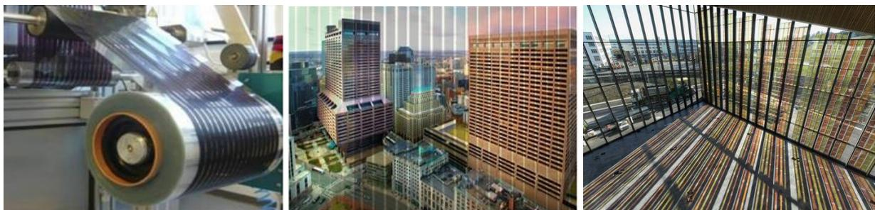
**Figure 1.2: (Left) Roll of OPV solar cells processed by Frederic Krebs group [11], (Middle) Integration in windows of buildings, and (Right) Swiss convention centre with DSSC Glass.**
